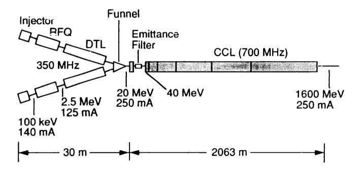
Fig. 1. Reference APT accelerator configuration
